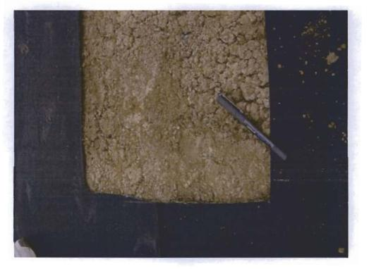
Photo 12: Desiccated Soil Subgrade at LE-1
